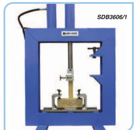
Shear test on wood
