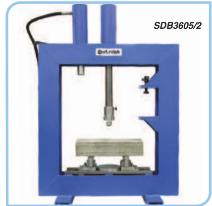
Test of flexion in 3 points
