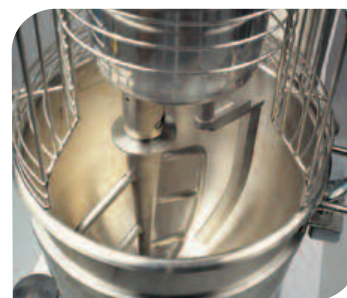
Scraper arm detail B0026/D
