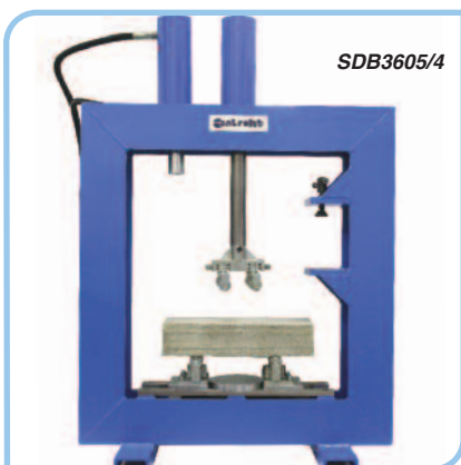
Test of flexion in 4 points
