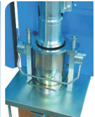
Detail of mould fastening system
