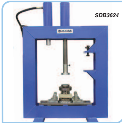
Test of flexion 4 x 4 x 16
